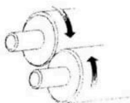
A missing cover can lead to a missing hand.
